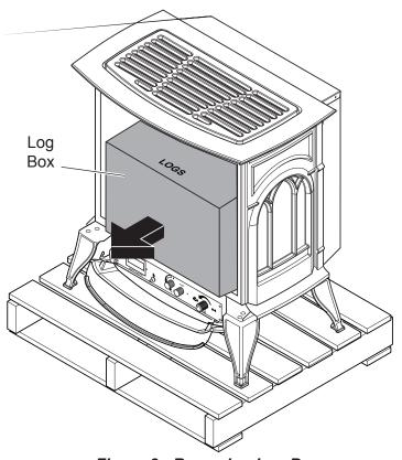
Figure 8 - Removing Log Box
